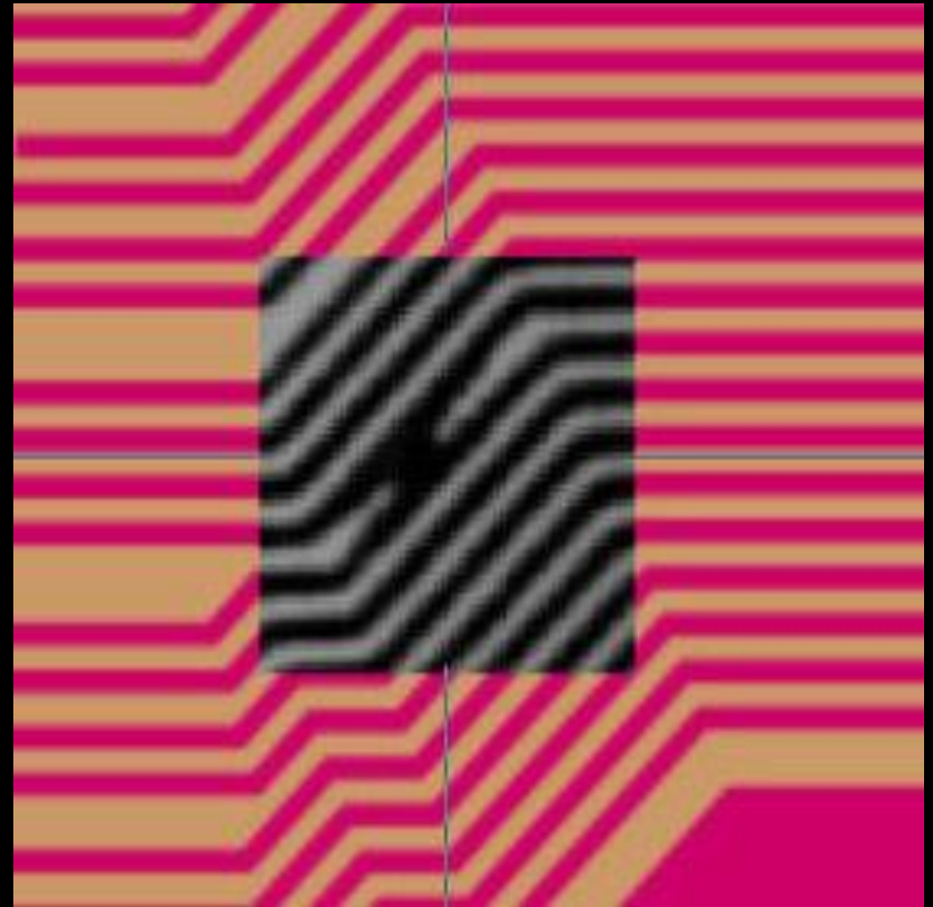
Scanned Image Superimposed Over CAD Data
