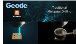
2. Geode begins drilling second via diameter without any tooling change
